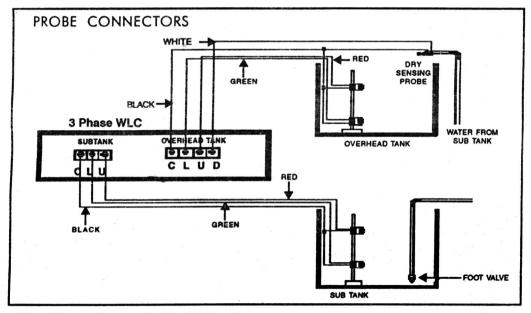
7. Your Videon 3 phase Automatic WLC is now ready for operation and the motor will be switched ON and OFF automatically in accordance with the water level conditions of both tanks.
